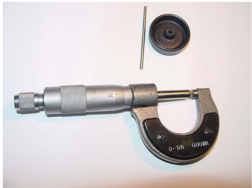
Figure 1 - Micrometer calipers with constant torque clutch next to a pin gauge of 0.0100" diameter used to calibrate the calipers for measuring bore-fitting drill bit shanks (not shown).
