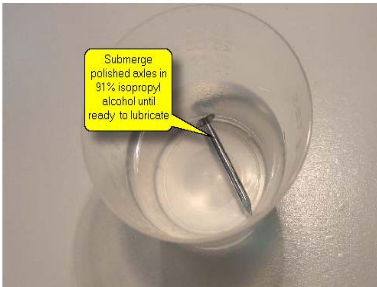
Figure 10 - Keep axle in a small cup of 91% IPA after polishing is complete.
