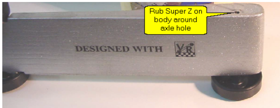
Figure 13 - Rub Super Z Graphite on body where wheel hub can rub.
