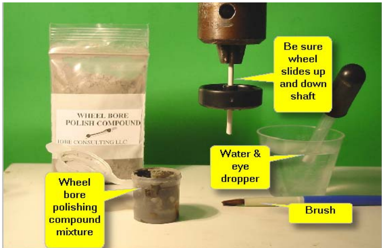
Figure 2 - Getting ready to polish the wheel bore.
