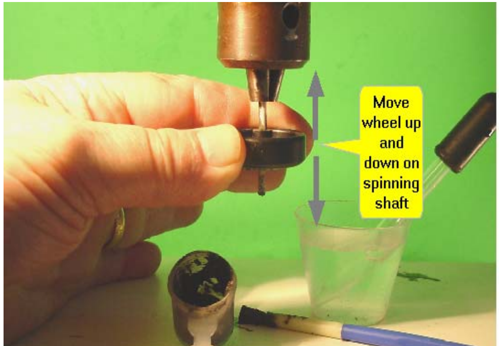
Figure 5 - Move wheel up and down a few times fairly quickly. If shaft hasn't swelled and tightened too much, flip wheel over and do a stroke through the other side of the bore.
