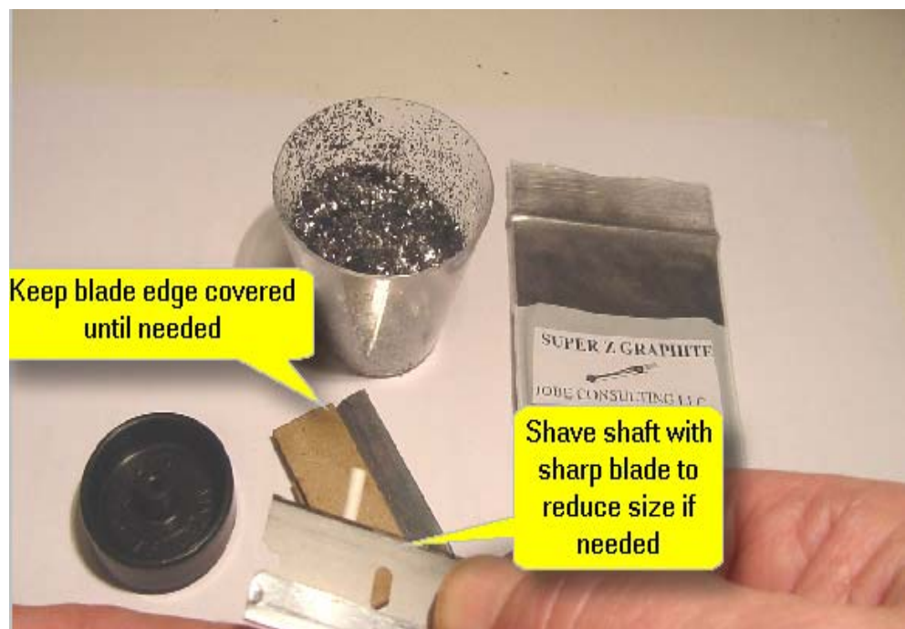
Figure 7 - If a cardboard shaft is slightly too large for the bore, it may be shaved down some with a razor blade (adults only).
