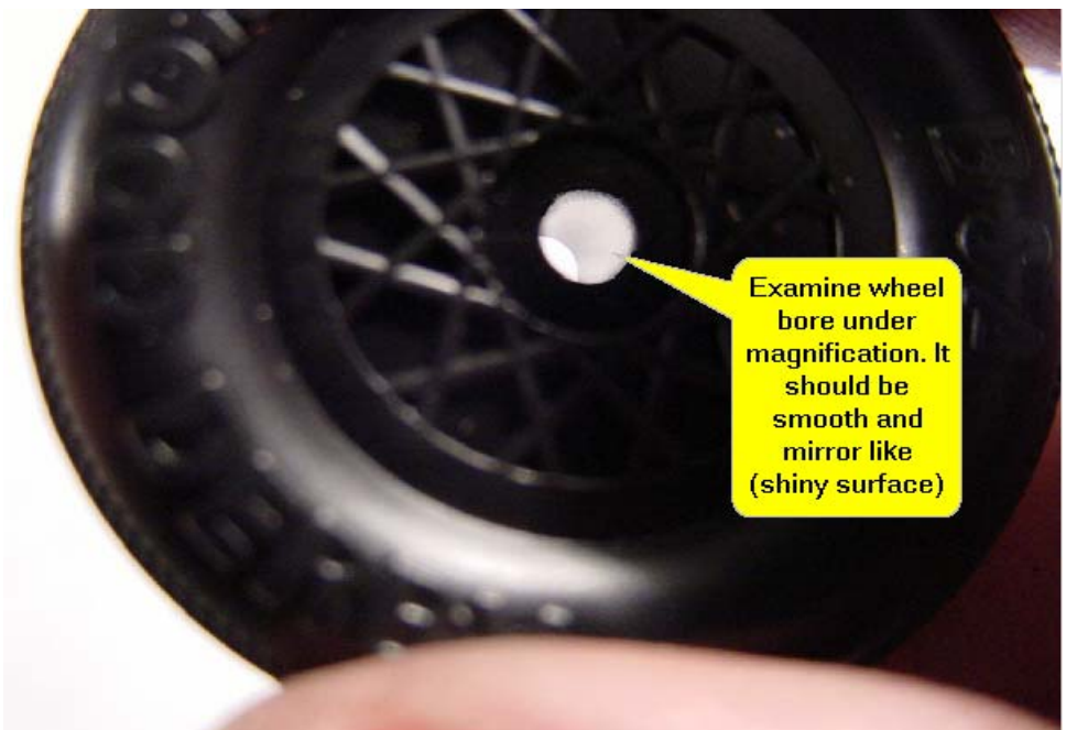
Figure 11 - Inspect the hub inside for smoothness and finish.
