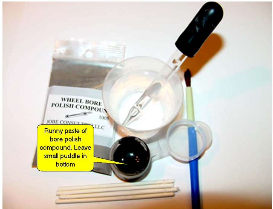
Figure 3 - Mix the wheel bore polish compound with a few drops of water to create a runny paste.
