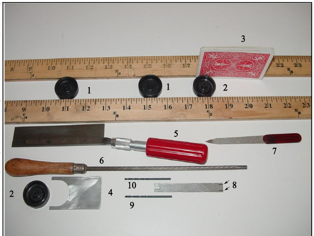
**Figure 9** - Wheel/axle measuring templates and related tools.
