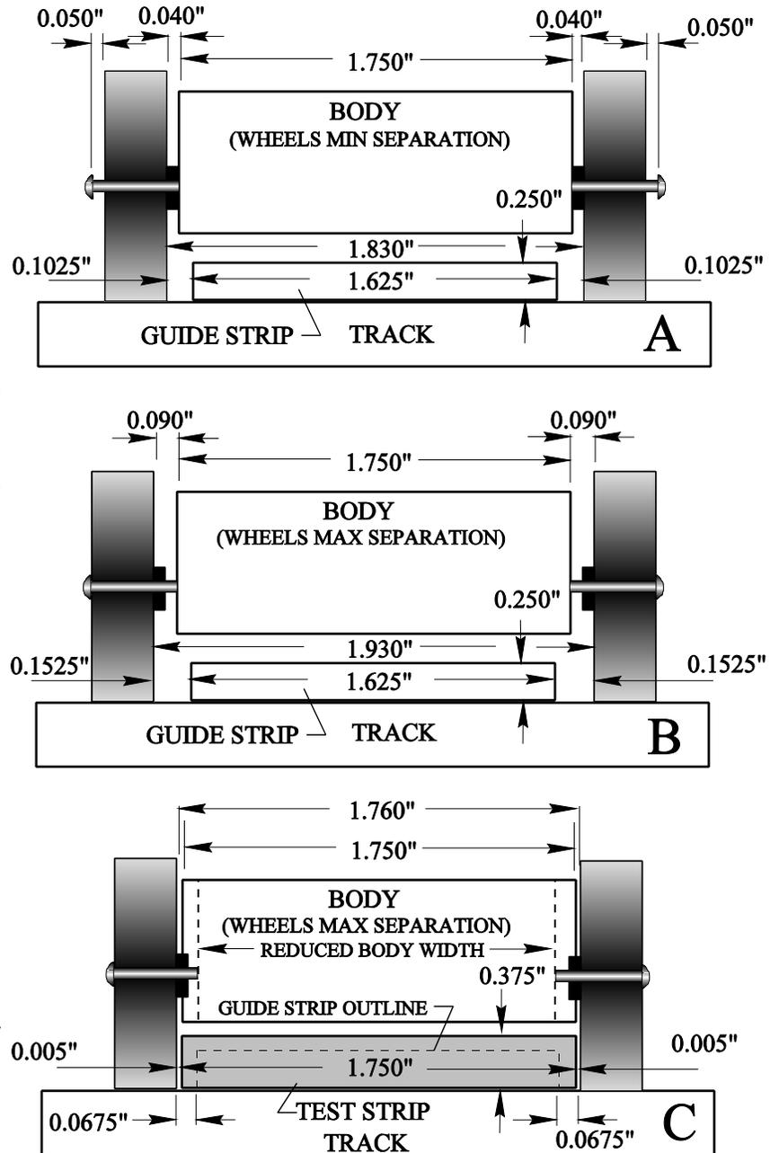
**Figure 6.** Measurements related to the 1-3/4" width rule.
