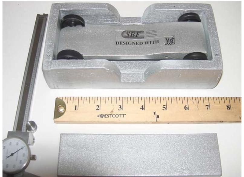
**Figure 8** - The car length and width box and the wheel clearance slab.
