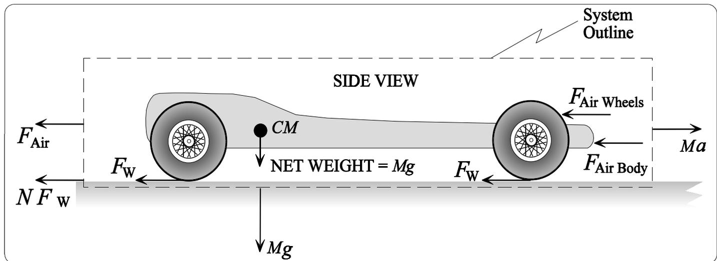
**Fig 7 - Forces associated with entire body plus wheels system.**
