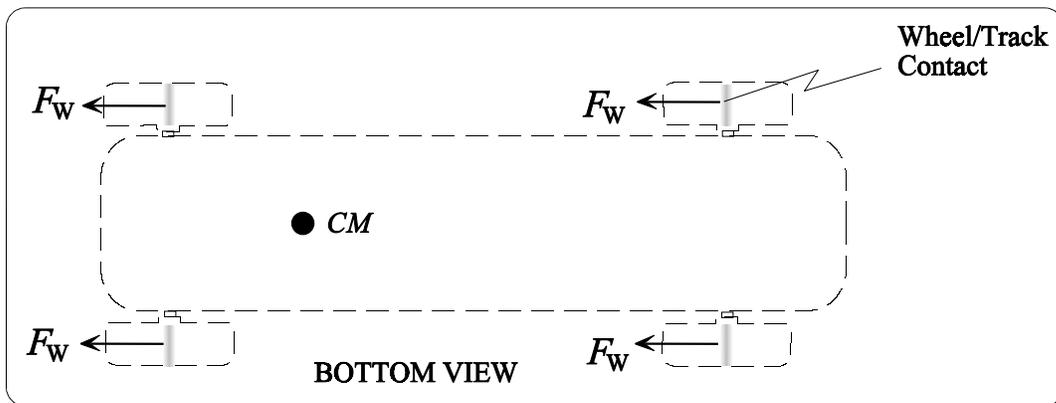
**Fig 8** - Forces where wheels tend to drag against track because of axle/bore friction.
