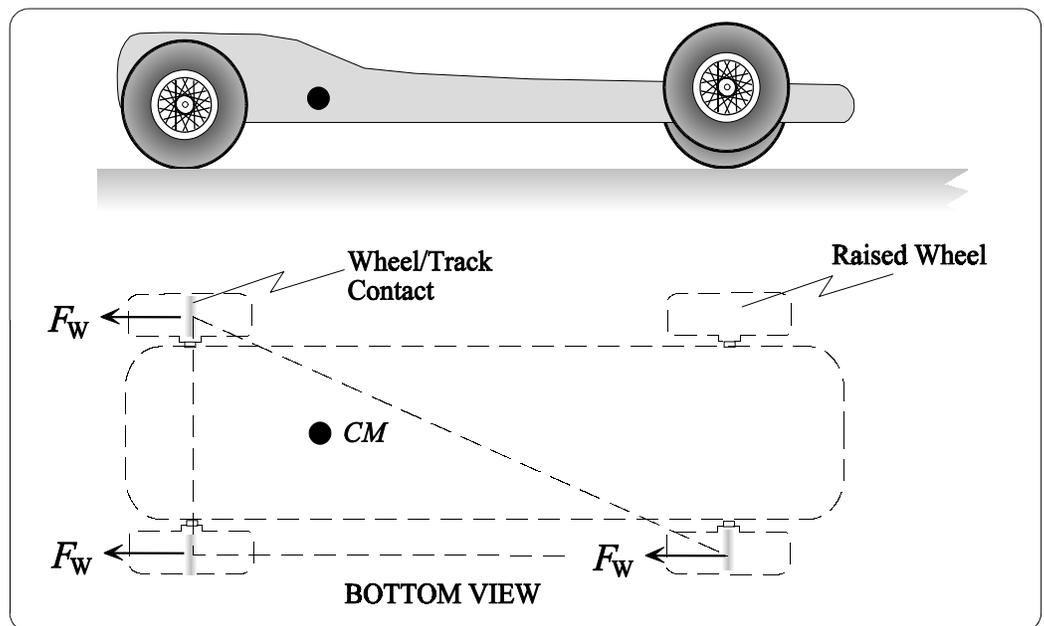
**Fig 9** - The case where one wheel is raised and only 3 wheels roll.
