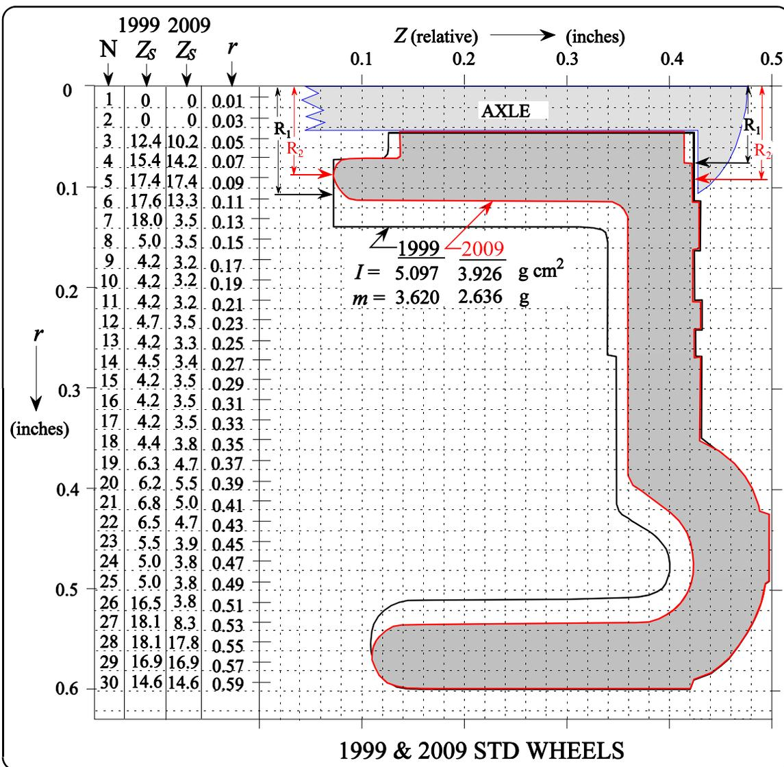
Fig 6 - Comparing the cross sectional changes in the 1999 and 2009 standard wheels. Zoom in this Adobe pdf page to get a better view.
