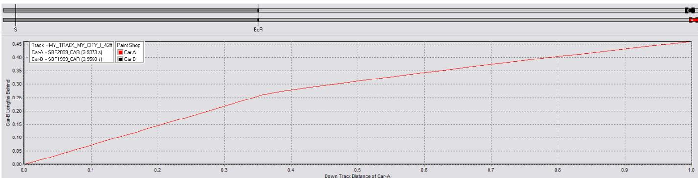
**Fig 8** - The SBF2009\_CAR ramp acceleration gives a 1/4 car length end-of-ramp advantage over its heavier wheeled twin and wins by almost half (0.459) a car length at the finish---Track is a 42 ft Best Track.
