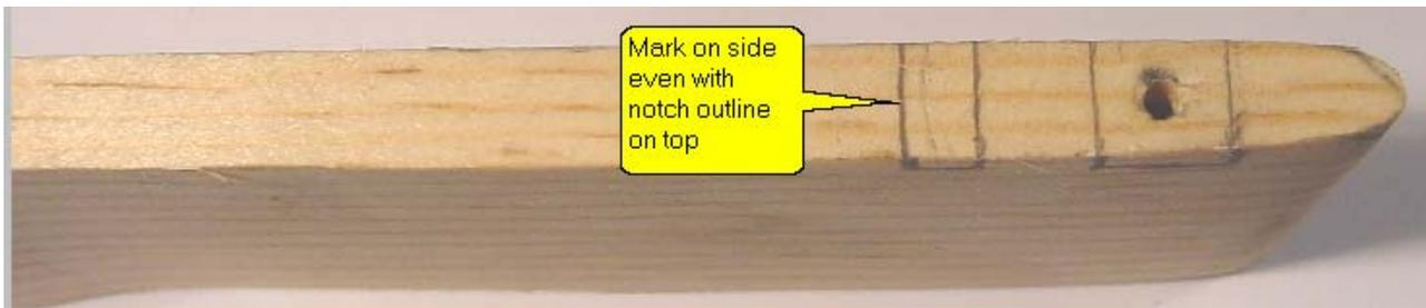
**Figure 20** - Mark notch edges on sides of car.
