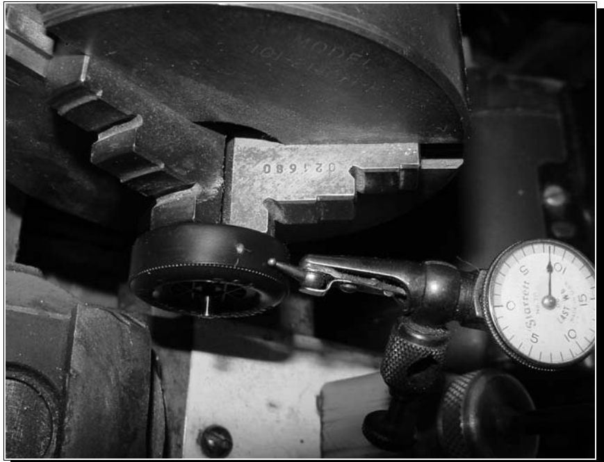
Figure 2 - Measuring amount of off-center on the wheel.
