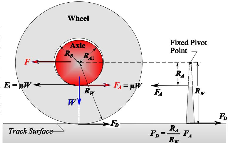
Figure 1. Forces on a wheel and axle.
