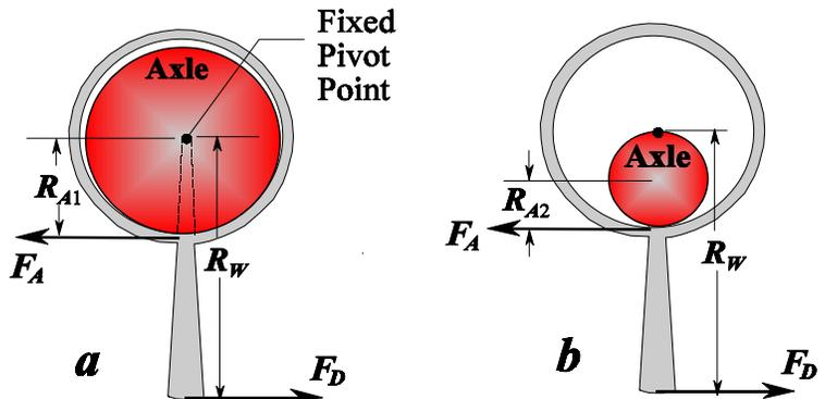
Figure 2. The wheel as a type 3 lever. Only wheel forces shown.
