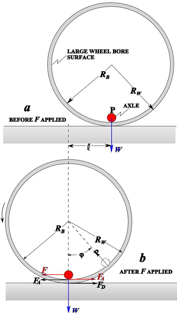
**Figure 3.** Showing a small wheel axle sliding inside a large wheel bore.
