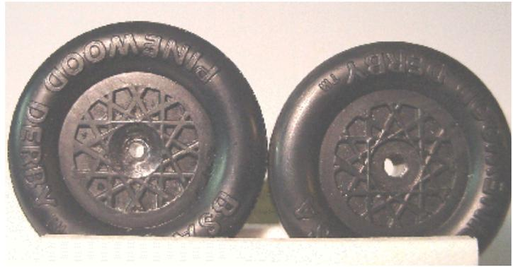
**Fig. 6.** Bores: Right standard. Left reduced using epoxy resin.
